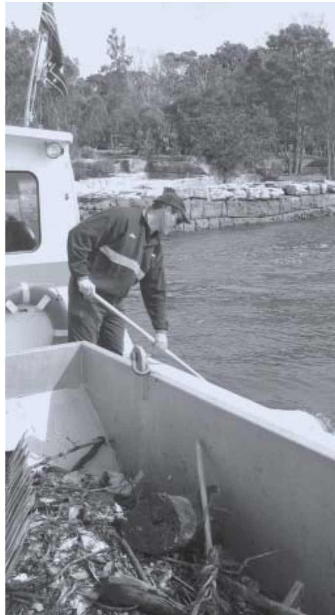
There are eight vessels in the Authority's purpose-built harbour cleaning fleet, the largest having a capacity of 28 cubic metres. Rubbish collected in Sydney Harbour is taken to Rozelle Bay where it is transferred to approved waste transfer stations
